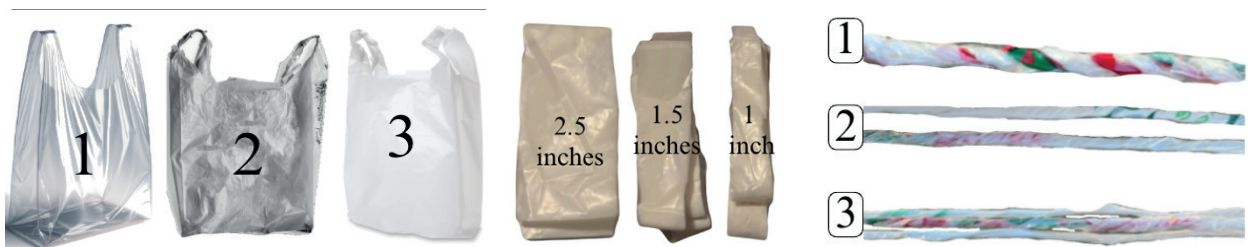
Figure 2. Material testing for plarn cord selection: bag types (left), strip widths (center), and twist configurations (right).
